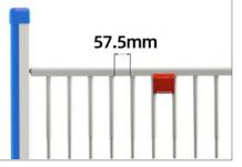
The gap between the railing is minimized to under 60mm to avoid entrapment of both heads and hands.
